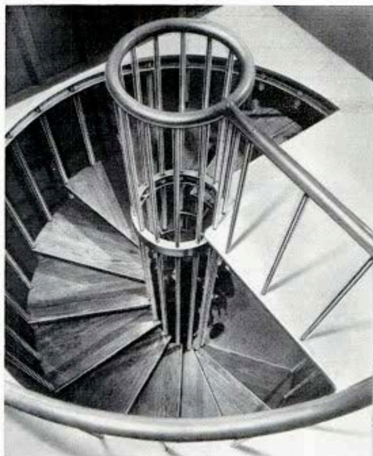
THIS IS THE SPIRA-STAIR. Suspended from a structural steel ring assembly, it is independent of walls for support. Spacing of gold anodized aluminum tubes eliminates need for handrail
